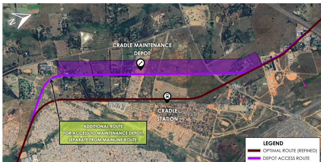
Figure 5-7: Optimal Location for Maintenance Depot at Cradle
